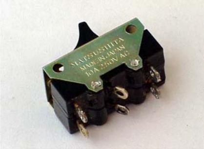
The contacts are heavy duty silver contacts, and with a cardboard strip, and some contact spray, everything is cleaned easily. Clean the contact by no means with a file, that will surely destroy the switch, use a special burnishing tool, or very fine (waterproof 800) sandpaper, if the contacts are in a very pitted state. If something of the case breaks, you can repair it using quick bonding glue, but if you are more carefully than I was, there is no need for that.
