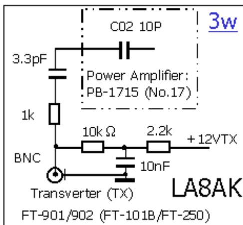
ohms in series (the resistor is used to avoid parasitics). About 20mW is available on 10M.
