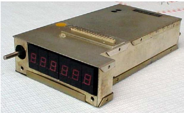
**Counter and display unit PB-1729A/PB-1730 (early model) , PB-2086A/PB-2098A (late model).**
