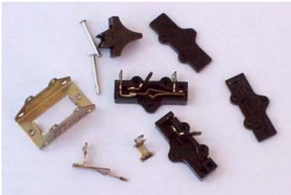
Assemble the switches in reverse order, and tap in the rivets carefully. Use a centerpoint or similar tool to close the rivet, just by pushing it by hand. Do not use a hammer, the material is too soft, and breaks away.
