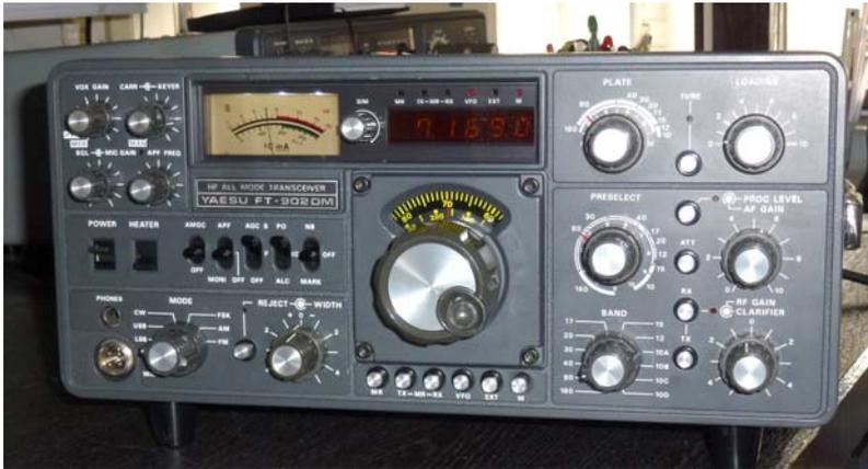
At the car I removed the cover, to see and smell if I could locate some recent burned parts, but to my surprise, the set was for its age inside very clean, even the fan had not much dust in it. Only the power switch was out and I could see that the switch has more or less disintegrated by a heavy current. It seemed that the set was a victim of a direct lightning stroke on the mains that is in parts of Belgium and France still with overhead cables.
