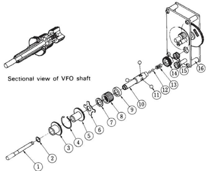
The exploded view of the gear displayed above is similar in build as the FT- series VFO gear.
