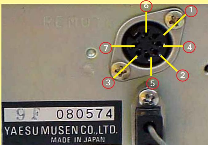
Yaesu used not the standard DIN numbering, so you have to check your voltages to be sure. I measured the connections shown above. The bandswitch supplies 12Vdc on the remote connector at the positions shown. This output can be used for switching antenna's, antenatuners or other band related equipment Use a low-current relay ca 100mA.
