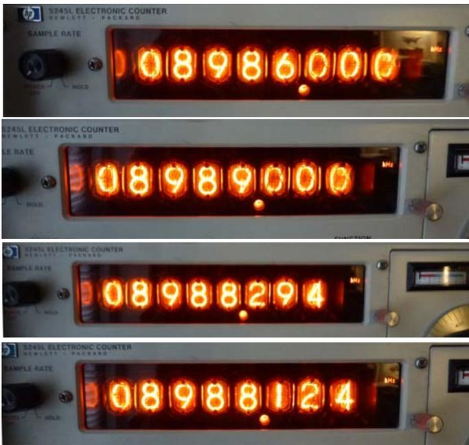
counter, both carrier frequencies are spot-on, even better than 2hz. After much headscratching I measured the MSM-9520RS out, (no documentation available) and found out that one of the preset ports was not working anymore, so I missed an offset of 2khz.
