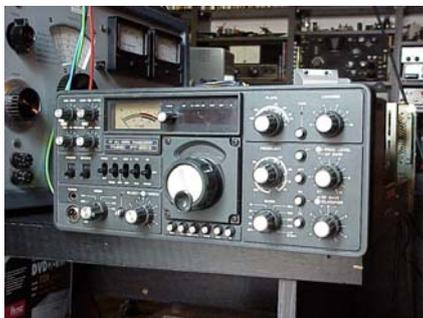
The meter says that I have a High Voltage of 850 Volts, there is no sizzling or other undesirable noises, but no reception either, just receiver noise with the audio full swing, no signals on 80 meters with a piece of wire. After connection of a antenna, still no signals. Test with the calibrator gives me S9+20 signals, so the receiver must be working, and the fault must be in the front end.
