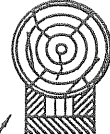
BOXING OF WOOD OF 1 1/2" MINIMUM THICKNESS. THE COVER IS TO BE NAILED TO THE SIDE PIECES.
